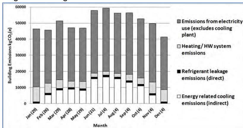
Figure 8. Monthly breakdown of building emissions
