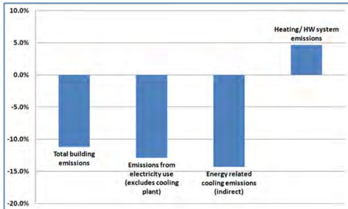
kgCO<sub>2</sub>(e) vs 15,300 kgCO<sub>2</sub>(e) for cooling emissions). The small increase in heating emissions is due to the reduced contribution from the lighting system to heating the building in winter.
