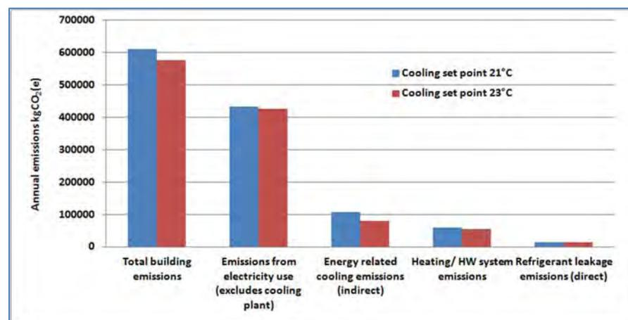
Figure 11. Impact of increasing the cooling temperature set point on cooling emissions
