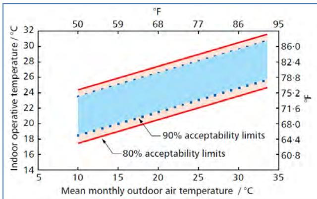
Opportunities may exist to reduce heating and cooling energy demand and emissions through adaptive control of temperature set points, according to the external environment. Figure 2 indicates that for any given outdoor air temperature there is a wide range of indoor temperatures that are considered acceptable by the majority of building users. Set points could therefore be adaptively moved near to these limits.
