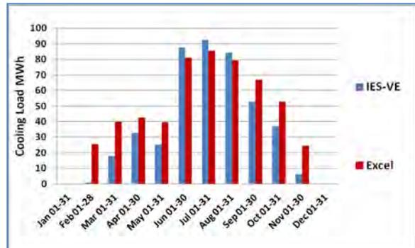
Figure 6. IES and Excel cooling load results
