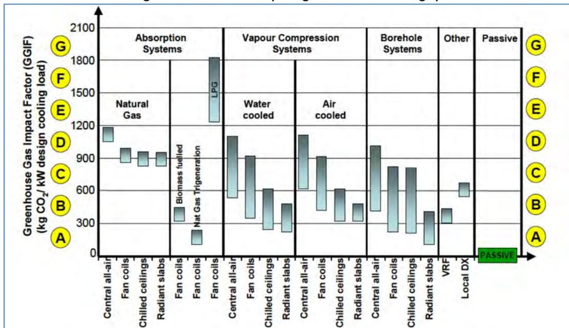
Figure 3. Greenhouse Gas Impact Factor and A-G ratings for typical modern cooling systems [8]
