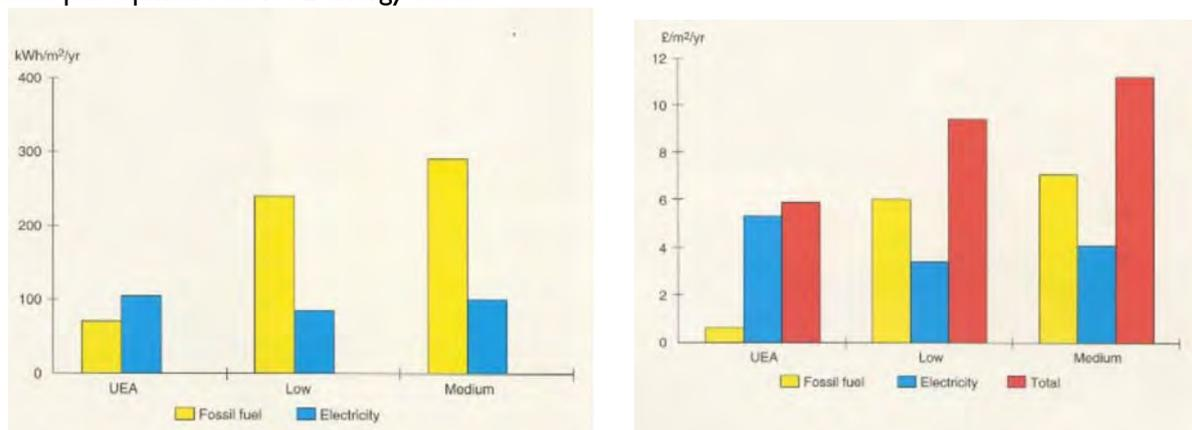
Figure 2: Annual fuel use (above) and energy costs (below) for Constable Terrace at UEA compared with the DOE's 'low' and 'medium' yardsticks for university residential buildings. [3]
