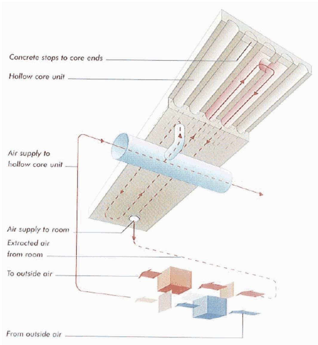
Figure 4: Diagram of ThermoDeck fabric thermal storage system [4].
