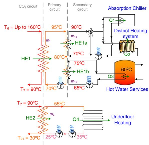
Figure 3: Schematic diagram of potential heat recovery systems
