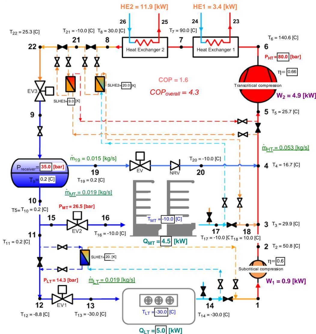
Figure 2: Conceptual design and EES model of novel system
